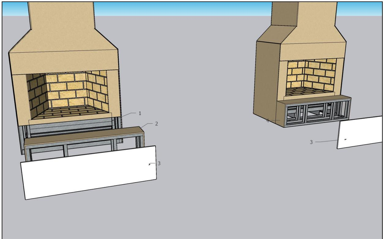
1. When fireplace (1) is set into position place hearth (2) in front of fireplace with the prefinished top up as shown in drawing.
